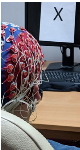
Fig.1. High Density electroencephalography (HD EEG) setup, including a cap and electrode sets, for recording the brain's electrical activity.
