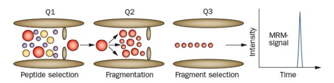
Workflow of an MRM analysis inside a triple quadrupole mass spectrometer. Abbreviations: MRM, multiple reaction monitoring; Q, quadrupole
